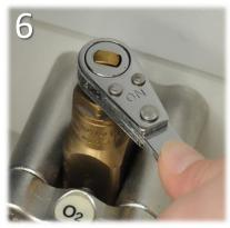
Turn the cylinder on using the spindle key. With the 'ON' surface facing up make two slow turns. Check that the cylinder is full by checking the gauge.
