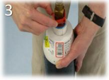
Remove the red plastic from the neck of the oxygen cylinder.
