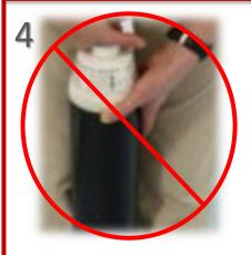
Do not hold the cylinder with your hands covering the holes on the neck. If there is grease or hand cream or alcohol on your hands this can be transferred. Mixing flammable substances with high pressure oxygen can be dangerous.
