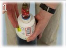
Hold the oxygen cylinder between your legs to prevent it from falling over.
